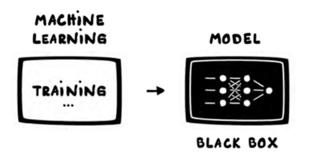
Identification of patterns in the input data via a statistical approach by the **learning** algorithm Creation of a new algorithm as result of the training process = **ML model**
